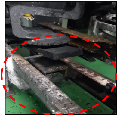
Heavy Paint deposition on wagon sprocket and hammerlock plate led to wagon rotation not ok phenomenon leading to defect
