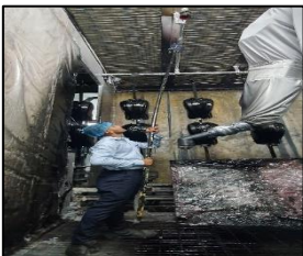
Frequent Cleaning of CO2 Pipe and Nozzle by stopping line (4-5 times/day) and Deep cleaning once/week
