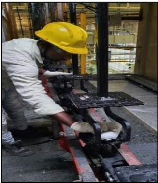
Deep cleaning of the complete wagon led to a reduction in indexing Not OK phenomenon elimination
